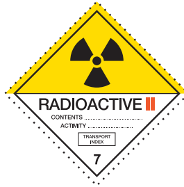
(No. 7B) Category II - YELLOW Symbol (trefoil): black; Background: upper half yellow with white border, lower half white; Text (mandatory): black in lower half of label: "RADIOACTIVE" "CONTENTS ..." "ACTIVITY ..."; In a black outlined box: "TRANSPORT INDEX" Two red vertical bars shall follow the word "RADIOACTIVE";
