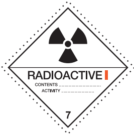
(No. 7A) Category I – WHITE Symbol (trefoil): black; Back- ground: white; Text (mandatory): black in lower half of label: "RADIOACTIVE" "CONTENTS ..." "ACTIVITY ..."; One red bar shall follow the word "RADIOACTIVE"; Figure "7" in bottom corner
