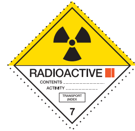
(No. 7B) Category II - YELLOW Symbol (trefoil): black; Background: upper half yellow with white border, lower half white; Text (mandatory): black in lower half of label: "RADIOACTIVE" "CONTENTS ..." "ACTIVITY ..."; In a black outlined box: "TRANSPORT INDEX" Two red vertical bars shall follow the word "RADIOACTIVE";
